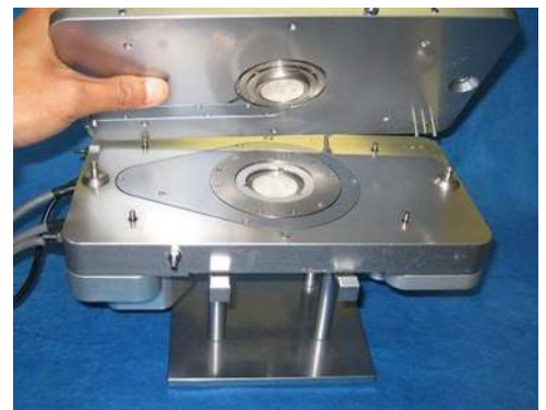
Lid of CSS450 being lifted off to reveal sample loading area
