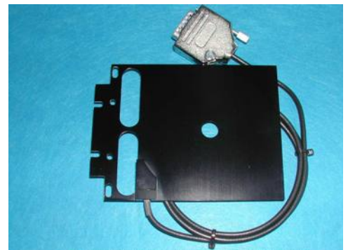
Fig 6 The THL series to fit onto the XY mechanical tables upright microscopes
