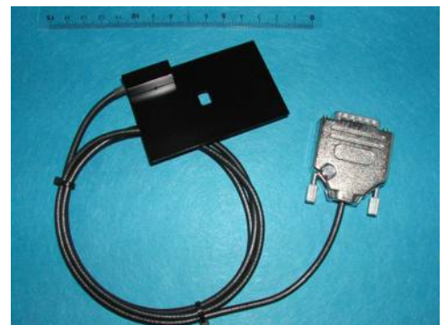
Fig 7 The TH series to fit into the slide holder arms of upright microscopes
