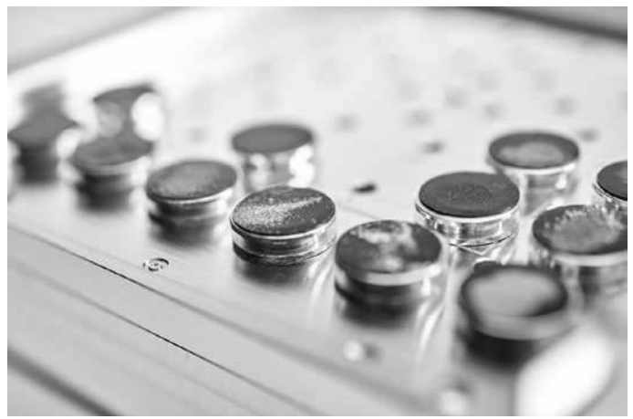
Sample holder with up to 30 x 12 mm pin stubs
