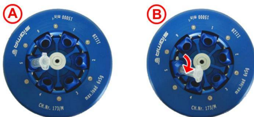
Fig. 8: Inserting big vessels
